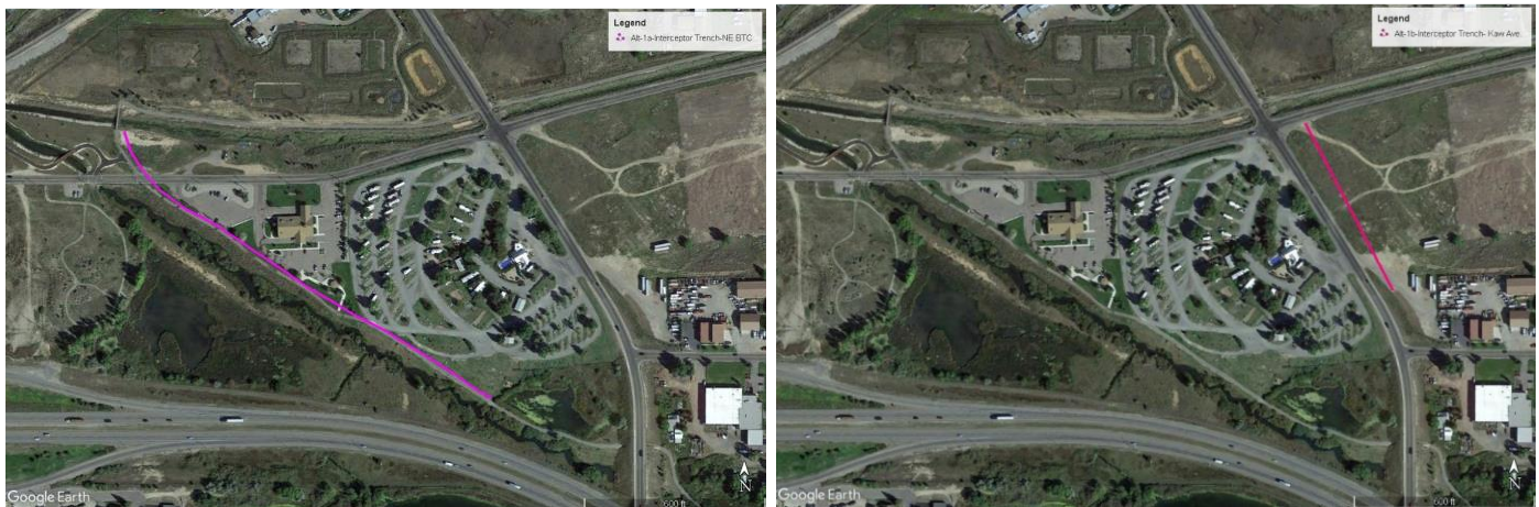
Images showing preliminary conceptual plans for either interception trenches or capture wells near Blacktail Creek
