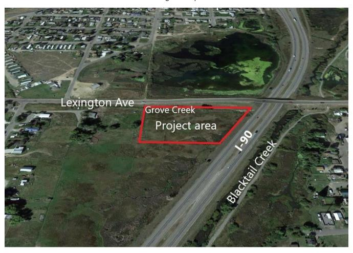
Metals from historic mining impact the Grove Creek watershed on the south side of Butte. The sedimentation bay provides water treatment by settling and adsorbing metals. Treated water will be released to Blacktail Creek which will benefit water quality and aquatic life in the creek. A rending of the Grove Gulch design from Atlantic Richfield's design is shown in the following drawing.
