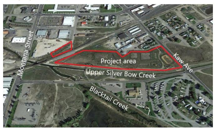
The Buffalo Gulch project will install multiple stormwater treatment basins and include trails and boardwalks for public use. The stormwater basins provide water treatment by settling and adsorbing metals and will benefit water quality and aquatic life in Silver Bow Creek. The images below provide renderings of the Buffalo Gulch project from Atlantic Richfield's design.
