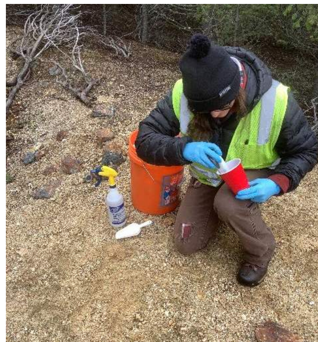
Sampling material from mine dump for field paste pH analysis
